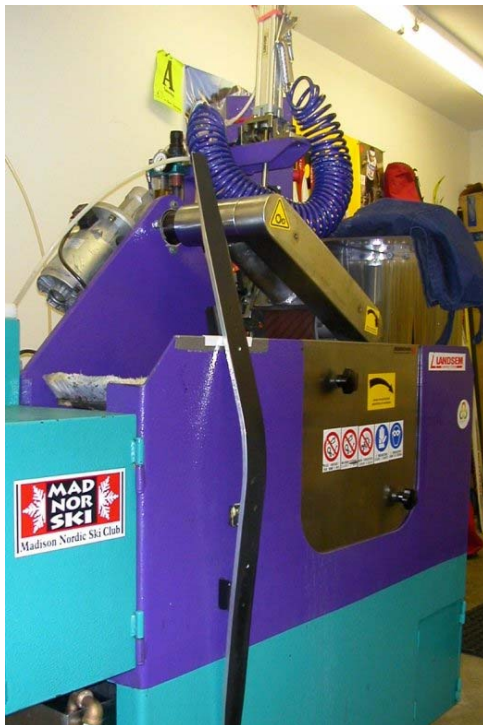
The Tazzari Grinder converts depleted p-tex into weapons grade ski bases!
